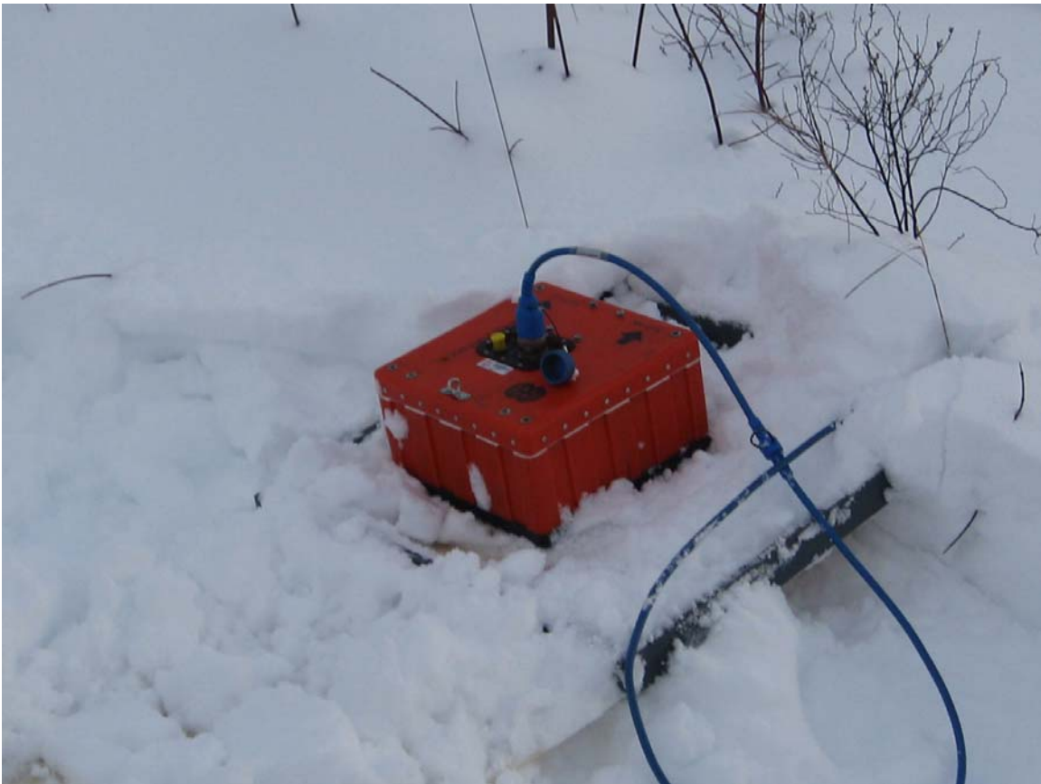
Figure 18. Ground Penetrating Radar 400 megahertz antenna on sled. (photograph by T. Fohl)
